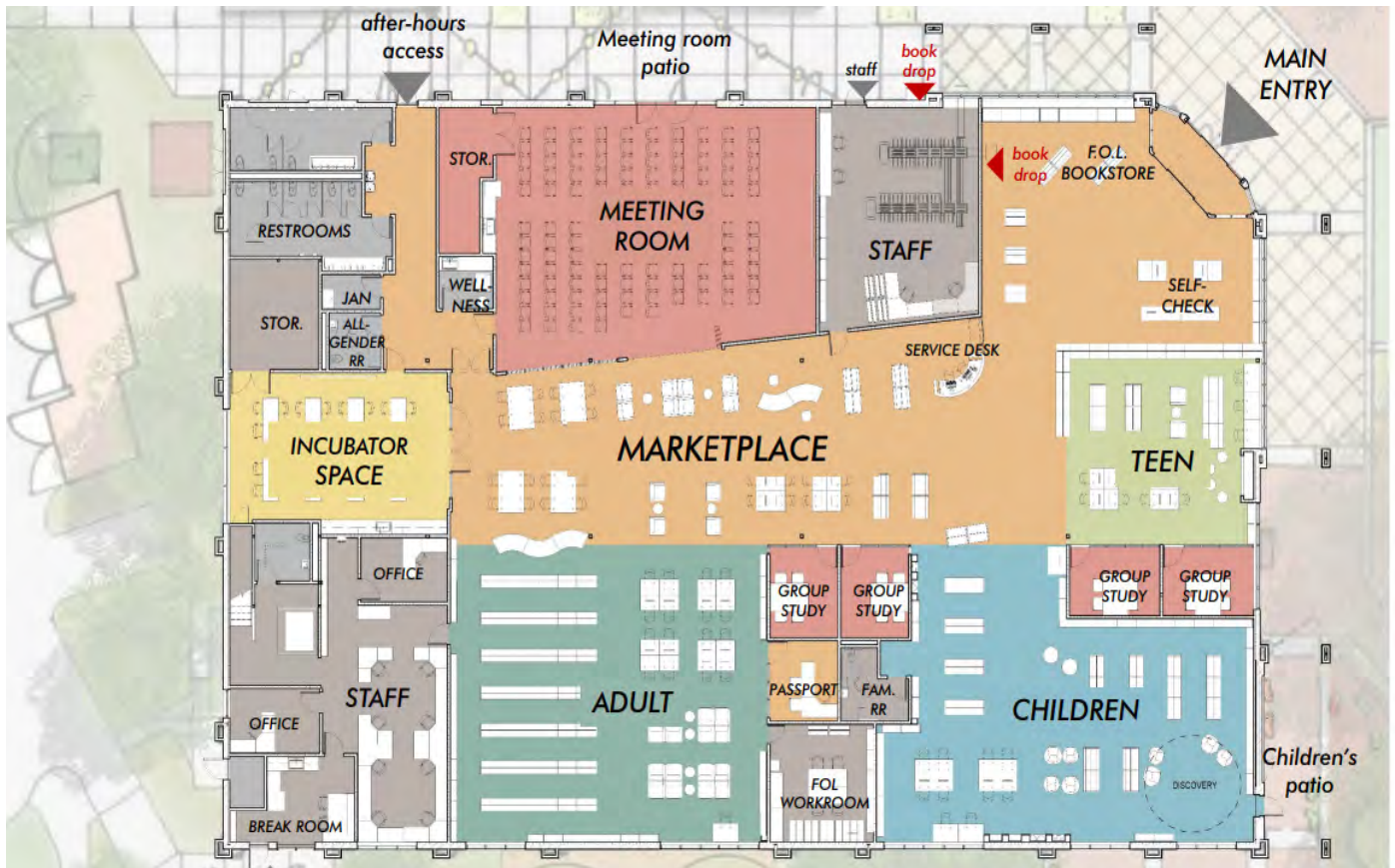
The draft floor plan for the new Elk Grove (East) Library incorporates large and flexible spaces for many library users and activities.
